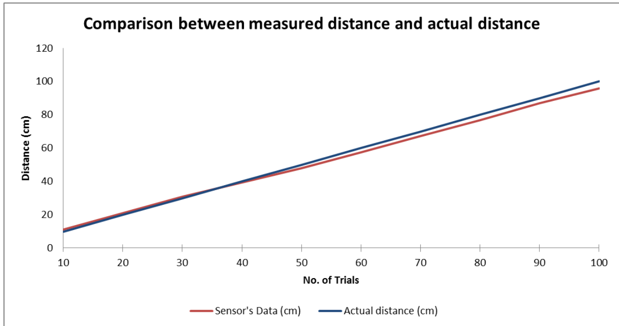
Figure 5: Variation between Ultrasonic sensor's measured distance and that on the ruler
